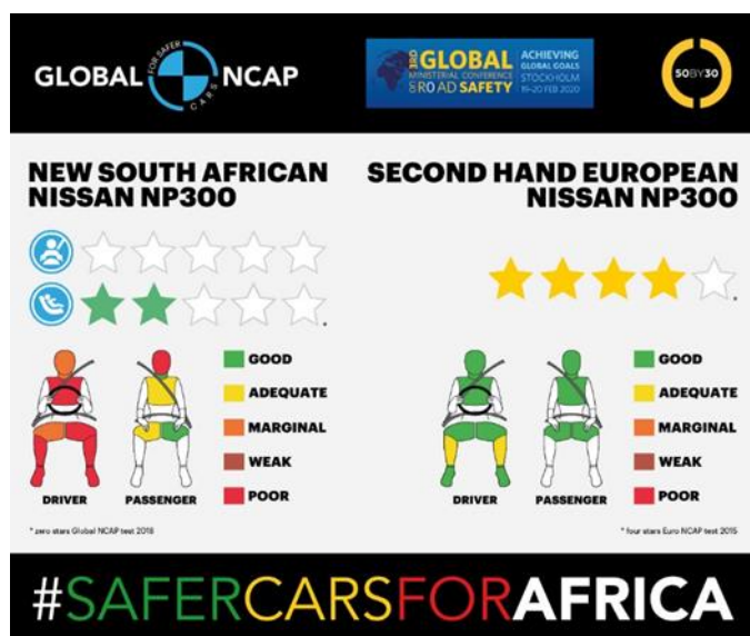
Figure 12: Diagram and safety rating comparison between Nissan NP300 Hardbody and Nissan Navara NP300 (Global NCAP, 2020)
