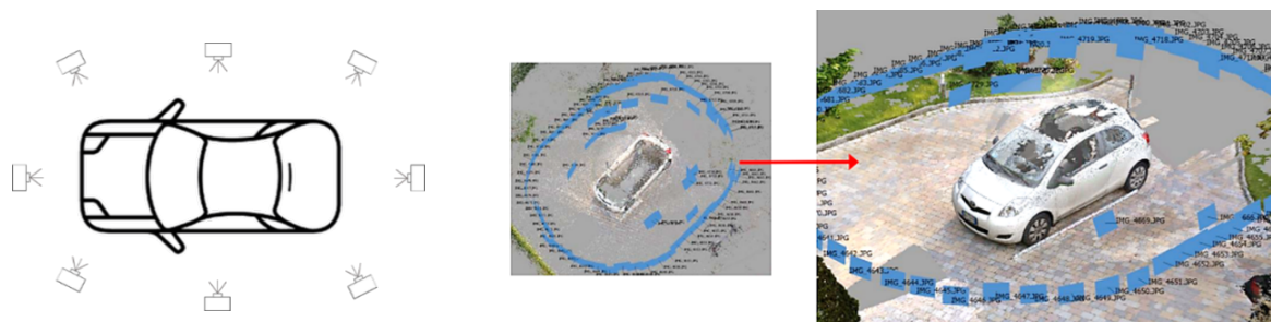
Figure 22 Exterior car photo angles (left) and a set of photographs for photogrammetry (right).
