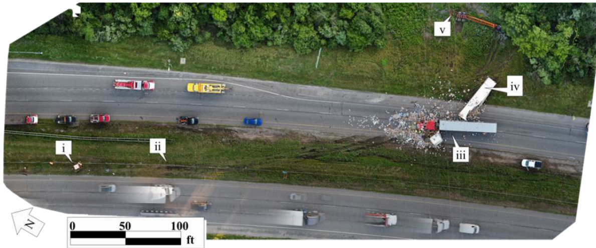
Figure 14 Scaled UAS ortho-rectified mosaic of an 8-min flight of a crash scene (Desai et al., 2022).
