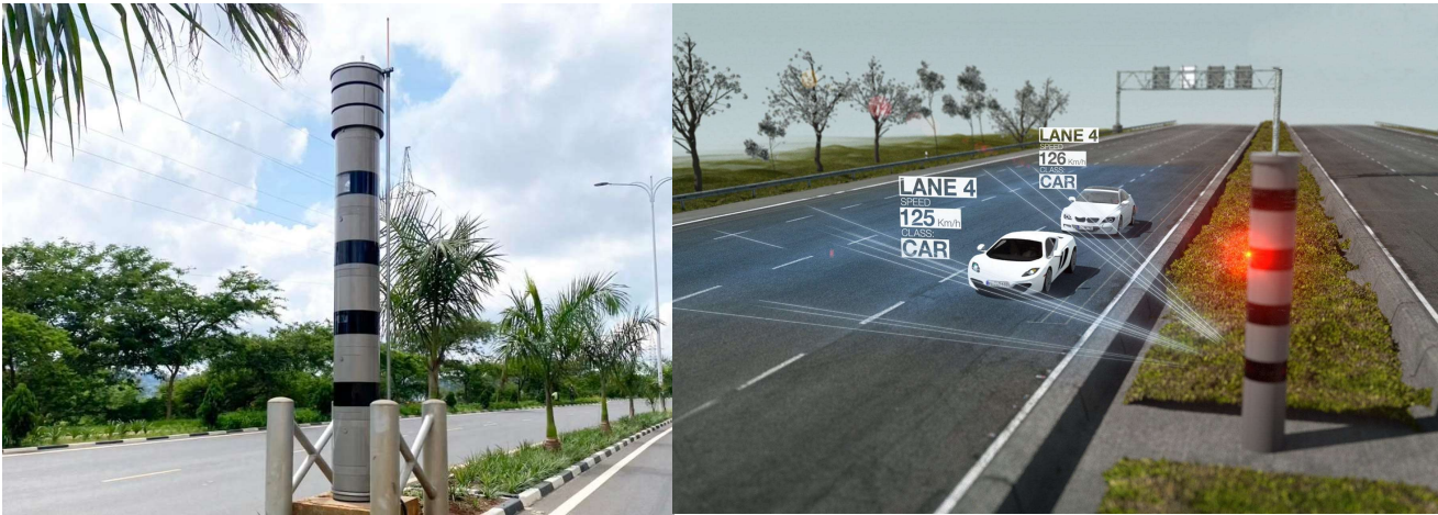
Figure 10: SSCs locally called as "Sophia" can monitor vehicle speed from multiple direction and numerous lanes using LiDAR for more precise speed measurement (Vitronic, 2023; Tabaro 2023)
